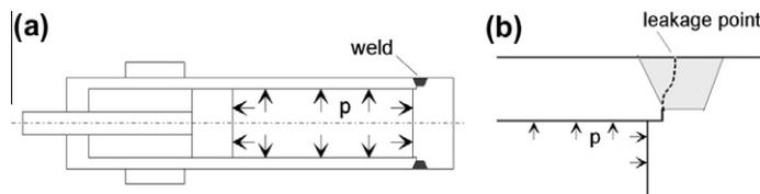
Fig. 1. (a) Scheme of the hydraulic cylinder; (b) detail of circumferential multi-pass weld and unexpected leakage location.
