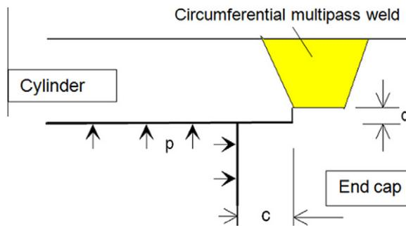
Fig. 2. Detail of the welded joint.
