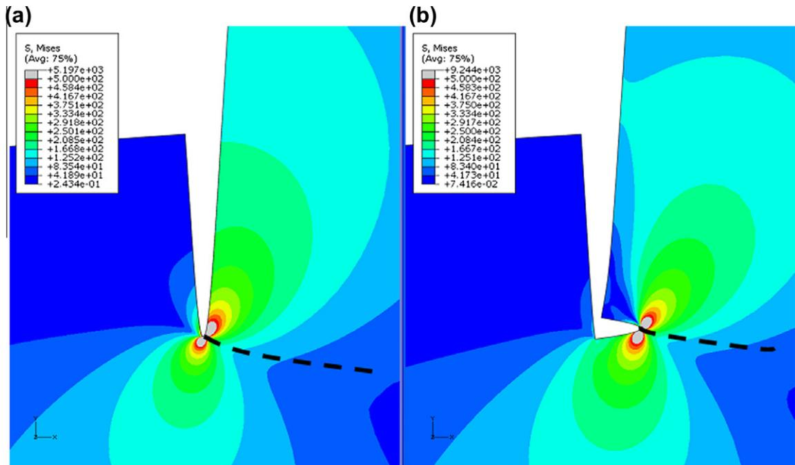
Fig. 3. Local deformation, elastic stress distribution and crack path for (a) V crack; (b) H crack. Scale  $\times 100$  (note that models are rotated  $90^\circ$  clockwise respect to Fig. 2).
