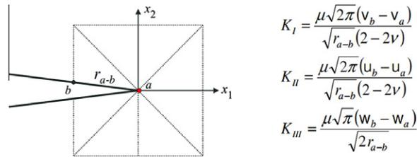
Fig. 4. (a) Node referred to the crack tip; (b) Mixed-mode stress intensity factors as a function of relative nodal displacements.
