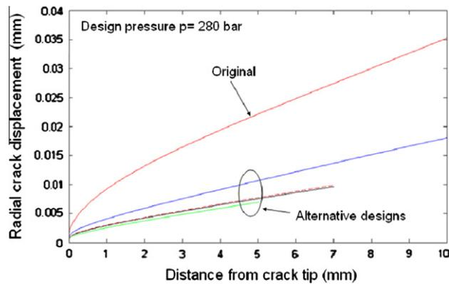
Fig. 7. Comparison of the opening displacement component of the original design and of alternative end cap designs.
