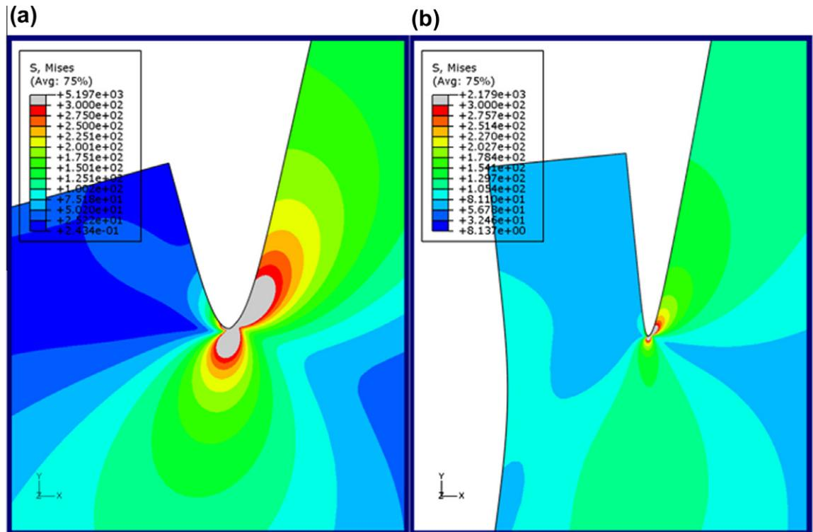
Fig. 6. Local stresses and deformation of (a) original cap design; (b) improved end cap design.
