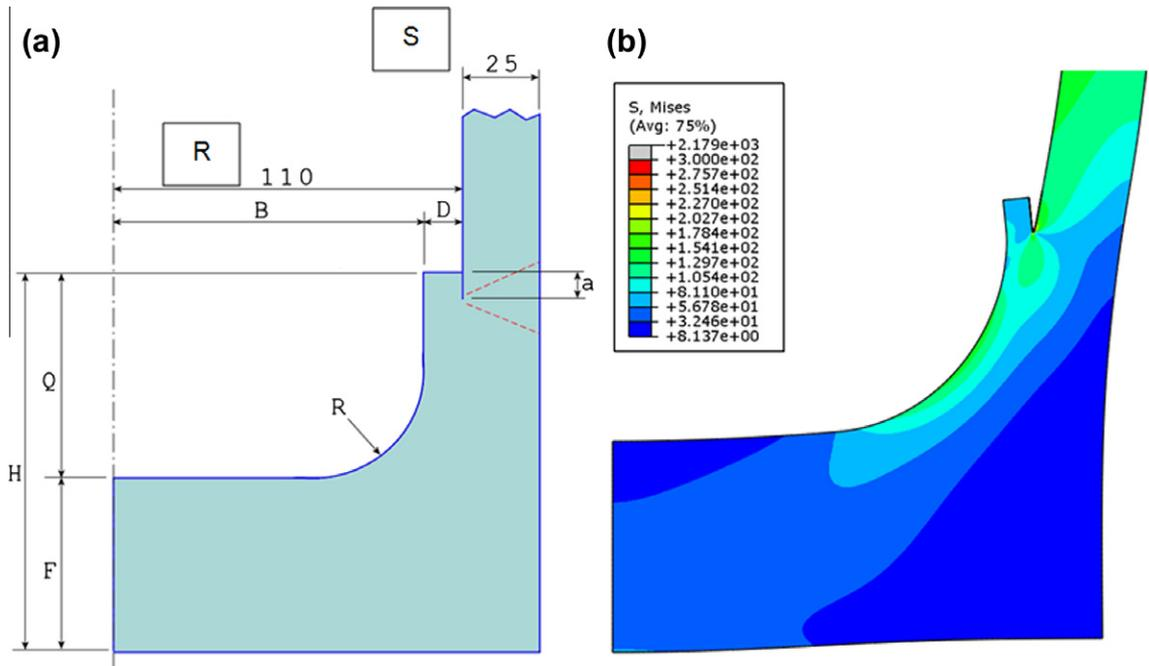
Fig. 5. (a) Modified end cap geometry with dimensions for parametric study; (b) elastic stress distribution for a configuration.
