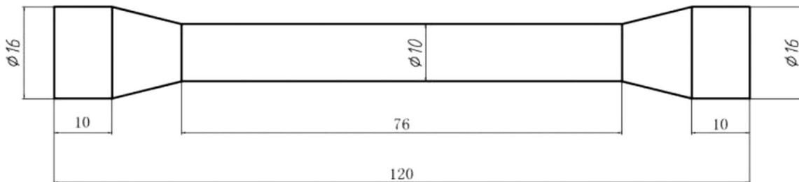
Fig. 6 2D figure of specimen
