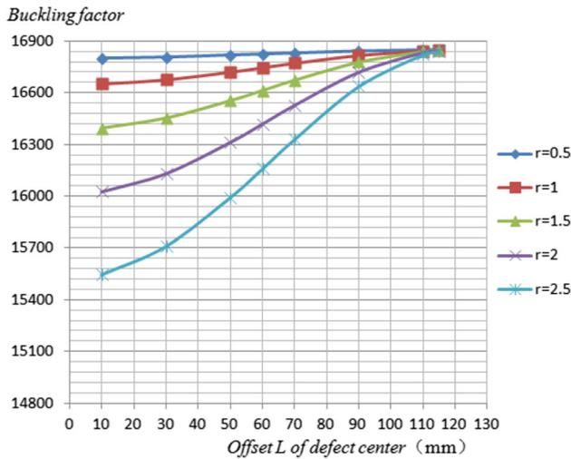
**Fig. 11** Buckling factor change with the radius of the defect. (a) Flap institutions of the power catwalk. (b) Hydraulic cylinder rod of the power catwalk
