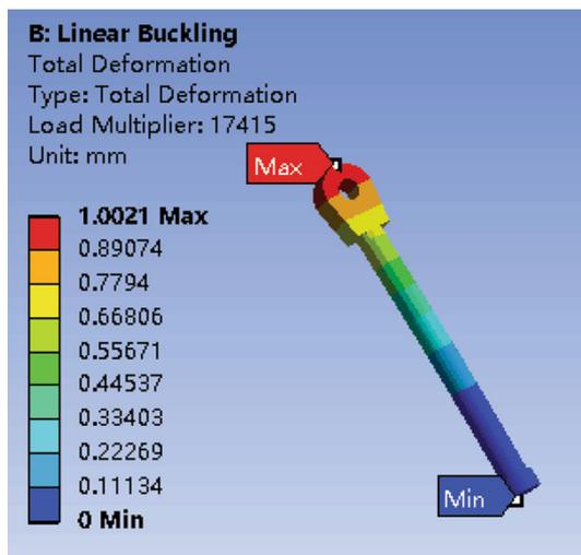
**Fig. 9** Buckling deformation diagram of hydraulic cylinder rod
