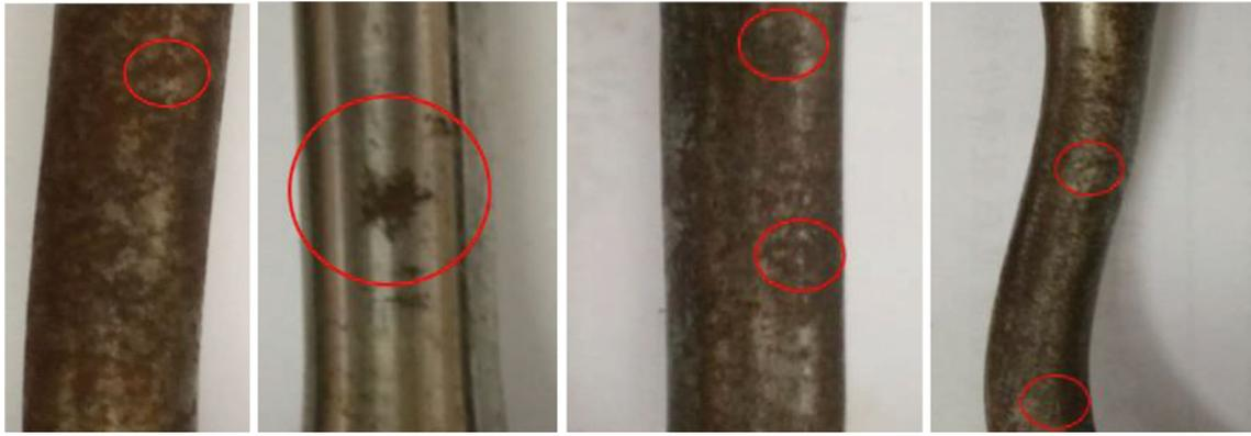
**Fig. 3** Defect in hydraulic cylinder rods after buckling
