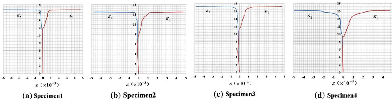
Fig. 7  $F - \varepsilon$  relationship diagrams of specimens. (a) Specimen1. (b) Specimen2. (c) Specimen3. (d) Specimen4
