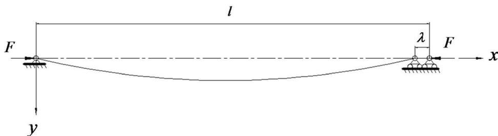
the moment of inertia  $I, I = \frac{\pi}{64}d^4, d = 10 \text{ mm}; l$  is 120 mm which is defined as the distance between the bottom and the center of the pin hole in the upper end of the hydraulic cylinder rod. According to mechanical design manual [22] and installation situation, the coefficient  $\mu$  is equal to 2. The  $\lambda$  needs to be quantitatively solved before solving the differential equation of the hydraulic cylinder rod.
