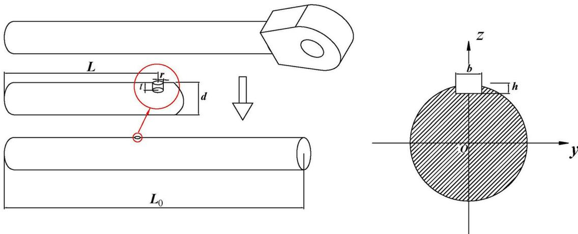
Fig. 4 Structure diagram of hydraulic cylinder rod with defect
