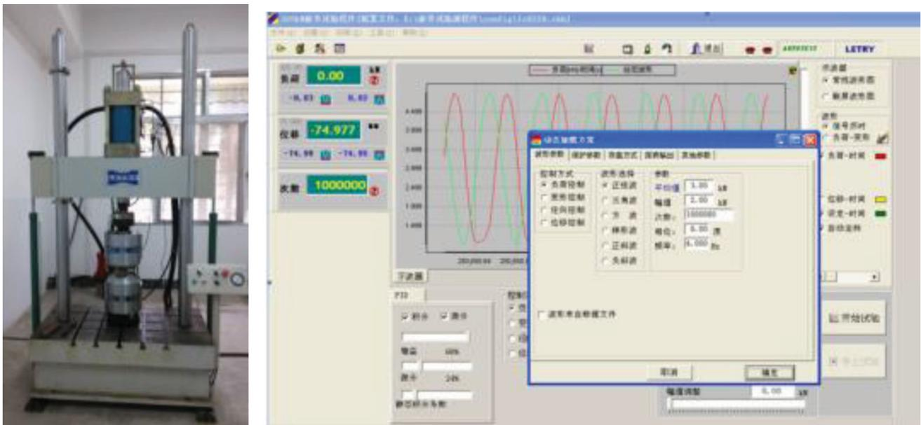
Fig. 5 Microcomputer-controlled electrohydraulic servo universal testing machine
