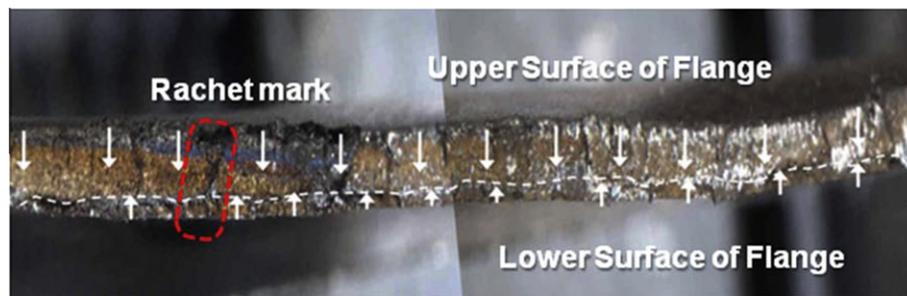
Fig. 4. Macroscopic investigation of the fracture surface.
