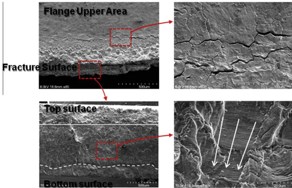
Fig. 5. SEM image of the upper surface and fracture surface.
