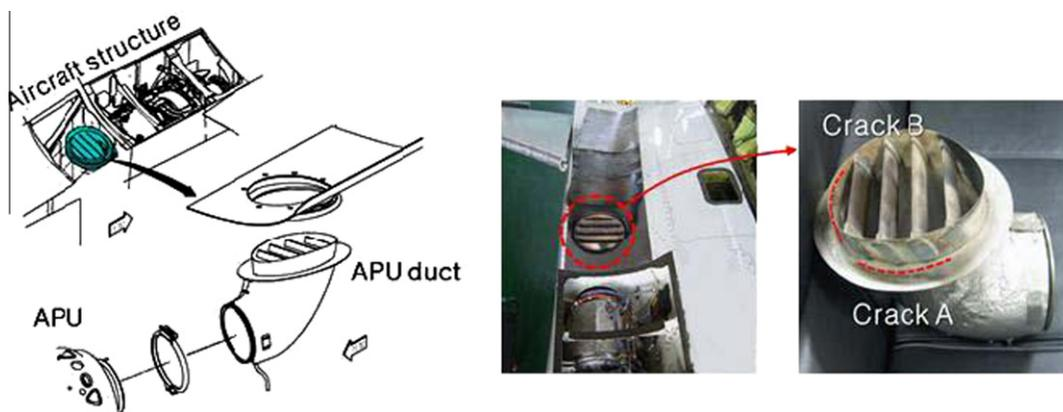
Fig. 1. Overall features of the APU exhaust duct.
