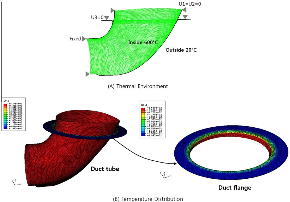
Fig. 8. Temperature profile of the APU duct (A) thermal environment and (B) temperature distribution.
