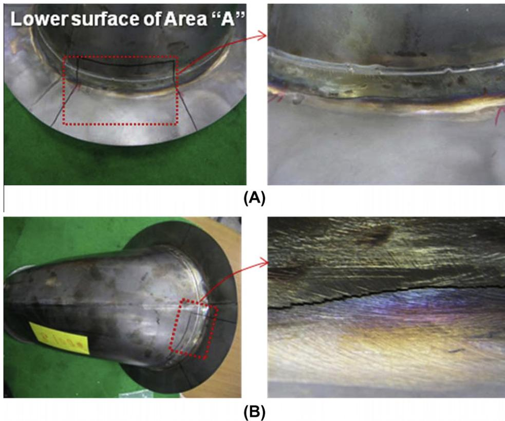
Fig. 3. Visual inspection of lower surface of the flange (A) discoloration and (B) scratches.
