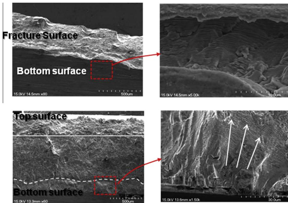
Fig. 6. SEM image of the lower surface and fracture surface.
