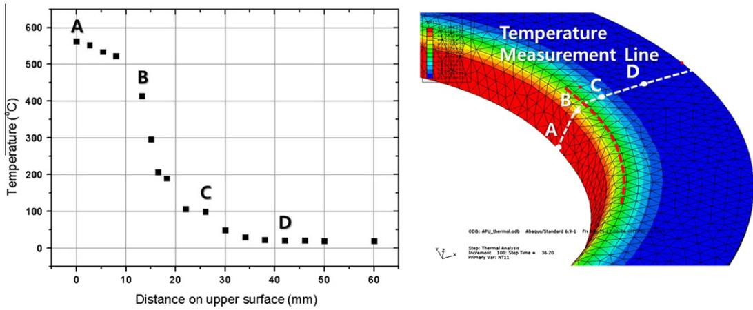
Fig. 9. Temperature distribution along the flange corner.
