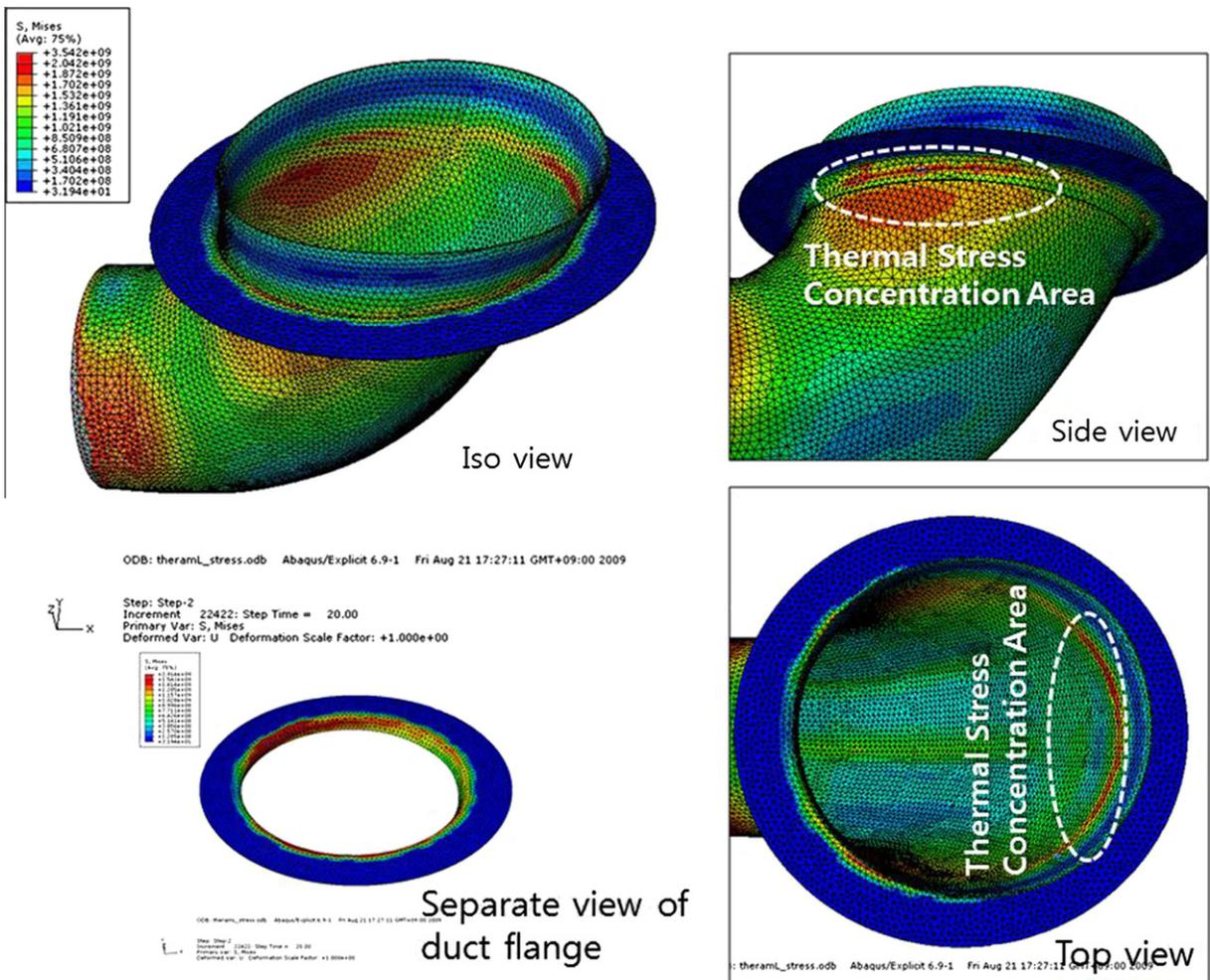
Fig. 10. Thermal stress distribution of the APU duct.
