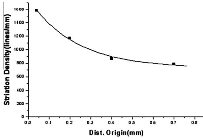
Fig. 7. Striation density of fatigue crack B.
