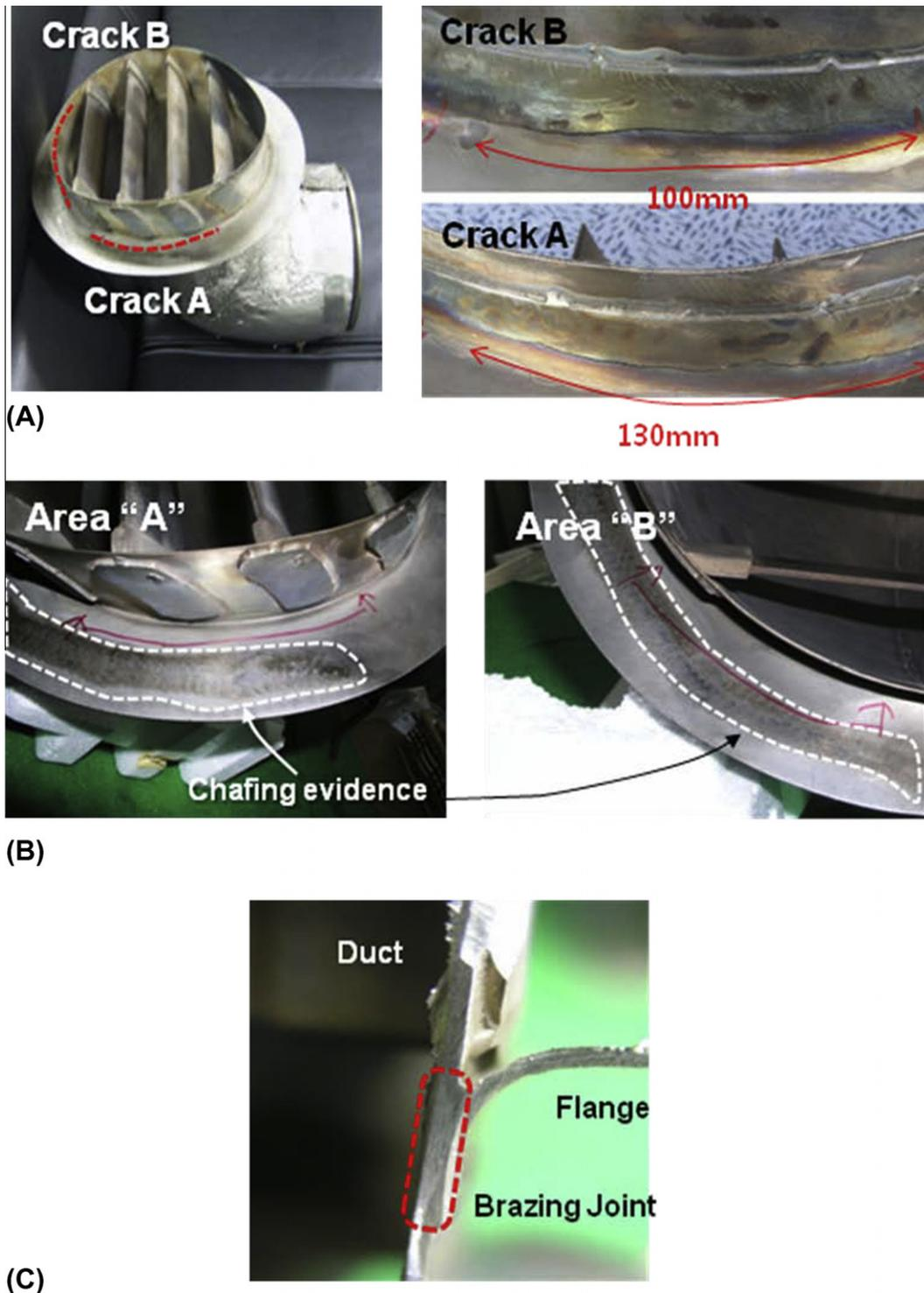
Fig. 2. Visual inspection of the failed duct (A) cracks, (B) chafing and (C) cut-away.
